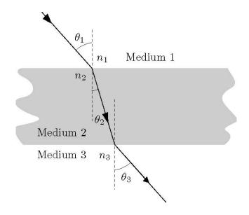
Figure 10.1: Double Refraction.
