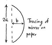
Dashed lines are normals (perndicular at 90° to) to mirror. All dashed lines intersect at the center. R is the distance from the center to any point on the mirror.
