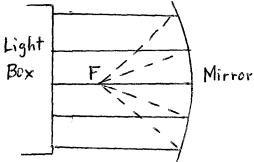
Compare your experimental value of f with theoretical value f=R/2, where R is the radius of curvature of the mirror. Trace the mirror on paper. This trace has the shape of an arc. R can be detrmined by either method:
