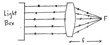
On the right side, all rays converge (intersect) at the common point F known as the "focal point" or "focus". The distance between the point F and the lens is defined as the "focal length" f. Measure and record this distance f and compare with the theoretical value:
